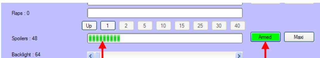
Now move the Spoiler Lever to it fully up position. See the indicator bar has now filled the box. Click the Maxi button to register the fully up position.
