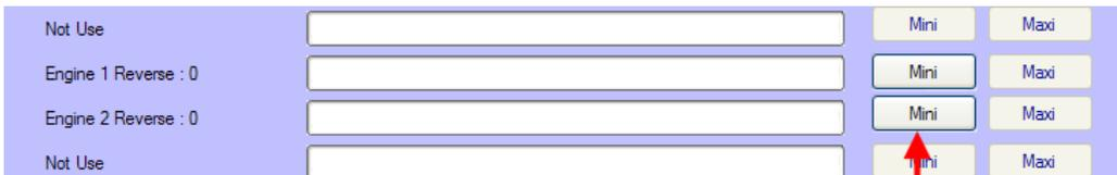
Move the lever to it's fully up position. You will see that the indicator bar has now filled the box. Now click the Maxi button alongside the Reverser 2 Indicator box.
