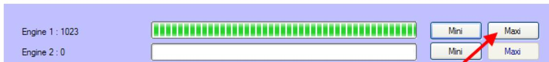
**REVERSER 1.** Raise the Reverse Lever Knob about 15mm from it's down position. This to ensure we return to a Zero Value when the Lever is down. Click the Mini button alongside the Reverser 1 Indicator Box. See also the note at the end of this document on Reversers.
