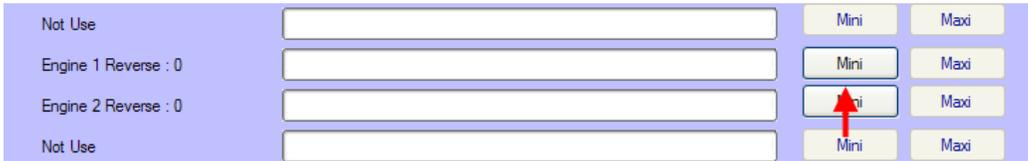
Move the lever to it's fully up position. You will see that the indicator bar has now filled the box. Now click the Maxi button alongside the Reverser 1 Indicator box.
