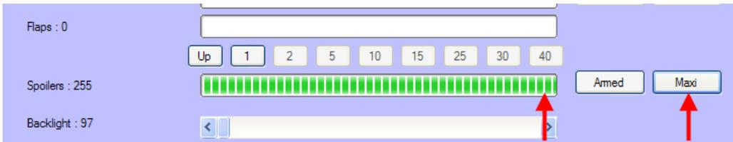
**FLAPS.** Place the Flaps Lever in the UP position. Click the button in the Configuration Interface window in the Flaps section that says Up.
